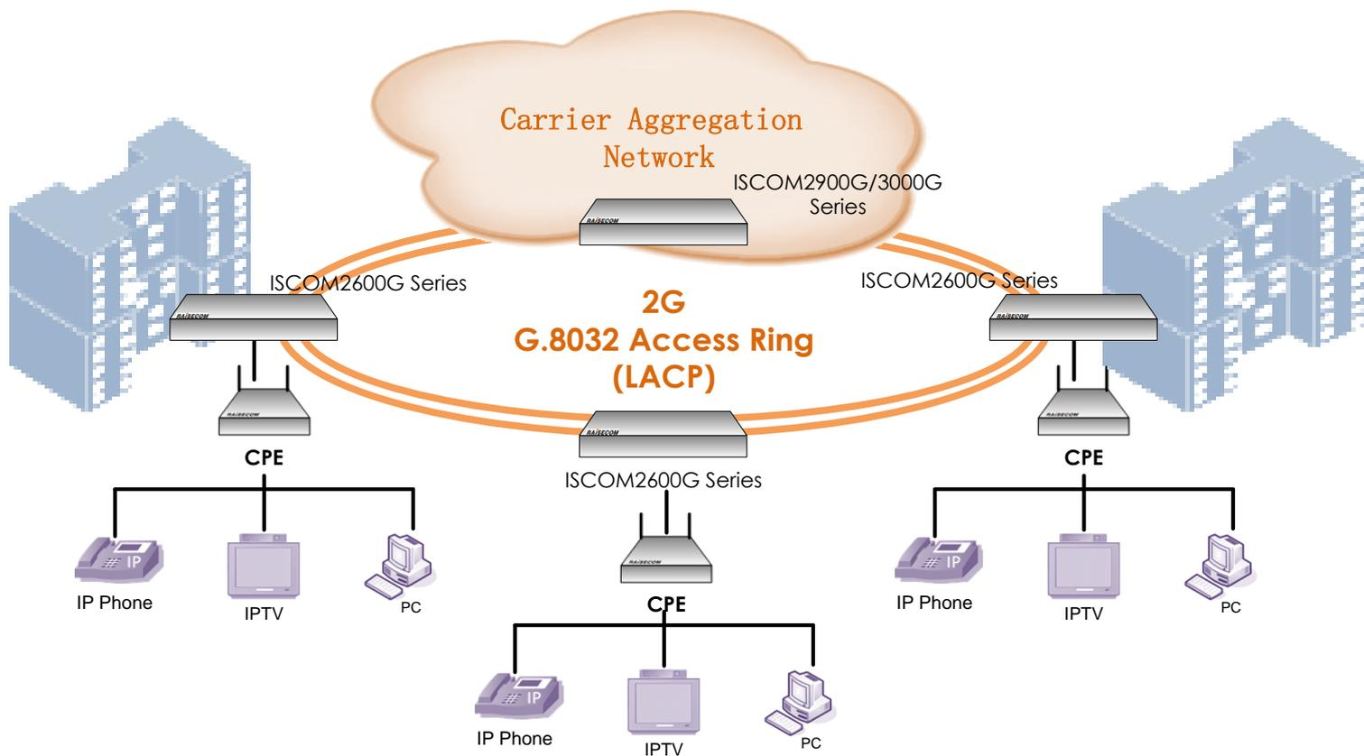
Figure.1 Application of the Gigabit access ring in the FTTH scenario
